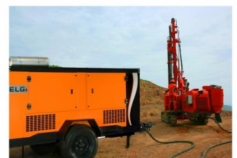
High pressure compressor for crawler drilling
